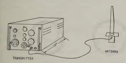
The sketch shows the pattern which might be seen on the face of the radar scope before and after jamming by means of random noises. Below it is a line drawing of a typical radar jamming transmitter widely used both aboard ships and in aircraft.
